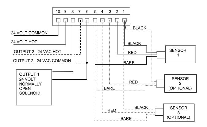
NOTE: When installing extra sensors, put all black wires to #1, all bare wires to #5, and red wires to appropriate positions. If sensor is installed as sensor 3, output 2 will operate on the temperature from that sensor instead of temperature from sensor 1 or 2.
