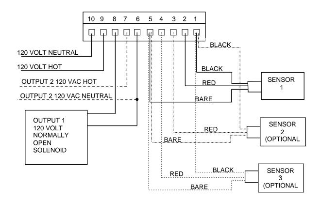
NOTE: When installing extra sensors, put all black wires to #1, all bare wires to #5, and red wires to appropriate positions. If sensor is installed as sensor 3, output 2 will operate on the temperature from that sensor instead of temperature from sensor 1 or 2.
